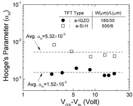
FIG. 8. Hooge’s parameters ( $\alpha_H$ ) vs  $V_{GS}-V_{th}$ .  $\alpha_H$  values are extracted from the linear region noise data ( $V_{DS}=1$  V) based on Eq. (26). Symbols (●) and (□) are  $\alpha_H$  values for a-IGZO and a-Si:H TFTs, respectively. Dashed lines indicate the average  $\alpha_H$  values.
