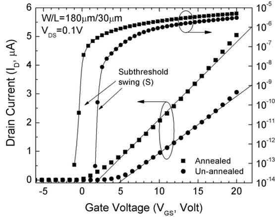
FIG. 2. Linear region transfer properties of rf sputter a-IGZO TFTs in semi-log (right Y-axis) and linear (left Y-axis) plots. Symbol (■) and (●) are experimental data for annealed and unannealed devices, respectively.
