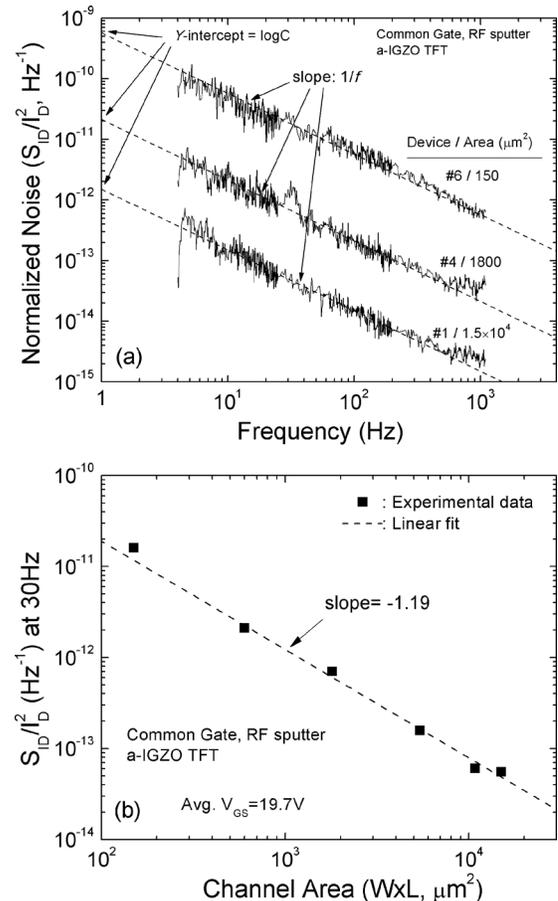
FIG. 4. (a) Examples of the normalized noise spectrums collected for three TFTs with different channel areas ( $150$ ,  $1800$ , and  $1.5 \times 10^4 \mu\text{m}^2$ ). Dashed lines are the best linear fits to Eq. (24). (b) Normalized a-IGZO TFT drain current noise [ $S_{ID}/(I_D)^2$ ] vs channel area. Data points (■) are sampled at  $30 \text{ Hz}$ . Dashed line is the best linear fit to the experimental data.
