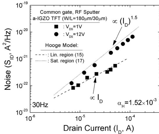
FIG. 9. Drain current noise power density ( $S_{ID}$ , sampling at 30 Hz) of the a-IGZO TFT as a function of drain current ( $I_D$ ). Symbols (■, linear region) and (●, saturation region) are experimental data. Dashed and dotted lines are calculated values based on Hooge  $\Delta\mu$  model.
