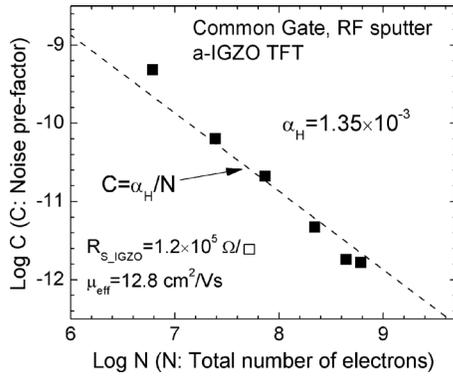
FIG. 5. Illustration of  $\alpha_H$  extraction based on area-dependent noise data. The total carrier numbers in TFT channel ( $N$ ) are calculated by Eq. (23) and are proportional to channel area. Noise prefactors  $C$  are numerically extracted from experimental noise spectrums as illustrated in Fig. 4(a). Symbol: experimental data; dashed line: suggested best fit to the Hooge model (25).
