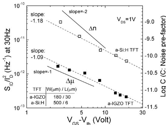
FIG. 6. Linear region ( $V_{DS}=1$  V)  $S_{ID}/(I_D)^2$  (at 30 Hz) and noise prefactor  $C$  as a function of  $V_{GS}-V_{th}$ . Solid (■) and open symbols (□) are experimental data for a-IGZO and a-Si:H TFTs, respectively. Dashed line: linear fit to the experimental data. Solid lines with slope of  $-2$  and  $-1$  are also provided for the aid of eye.
