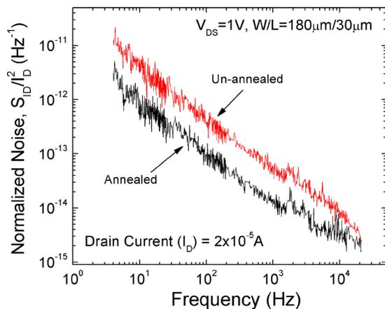
FIG. 11. (Color online) Normalized noise spectrums collected from annealed (black) and unannealed (red) rf sputter a-IGZO TFTs.
