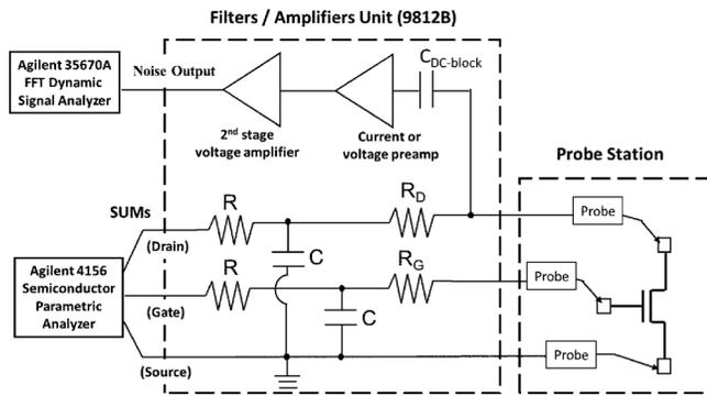
FIG. 1. Circuit diagram of the experimental setup used for measuring the TFT drain current noise. The filter/amplifier unit is also known as 9812B noise analyzer. (Adapted from Ref. 46). Device is placed inside the light-tight probe station, which also serves as a Faraday cage for electrical shielding.
