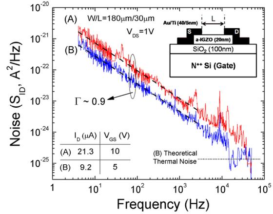
FIG. 3. (Color online) Example of a-IGZO TFT drain current noise spectrum ( $S_{ID}$ ). Two linear region noise data are shown ( $V_{DS}=1$  V). Data A (red) and B (blue) are measured under  $V_{GS}$  of 10 V and 5 V, respectively. (Inset) The cross section view of the common gate, rf sputter a-IGZO TFT used in measurements. (Dotted line) Thermal noise floor of condition B estimated from the theoretical model (2).
