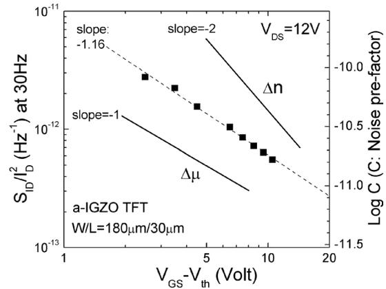
FIG. 7. Saturation region ( $V_{DS}=12$  V)  $S_{ID}/(I_D)^2$  (at 30 Hz) and prefactor  $C$  as a function of  $V_{GS}-V_{th}$ . Symbols: experimental data; dashed line: linear fit to the experimental data.
