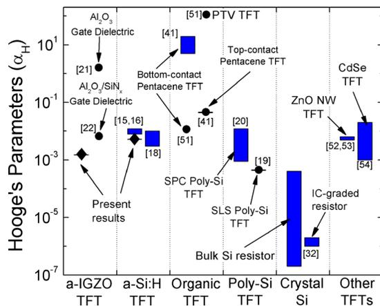
FIG. 10. (Color online) Hooge's parameter ( $\alpha_H$ ) extracted from the  $1/f$  noise measurement for various TFT technologies and crystalline silicon (data from Refs. 15, 16, 18–22, 32, 41, and 51–54, which are also indicated in the figure).
